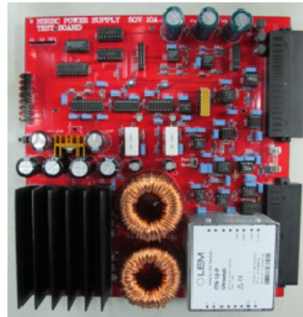
Figure 11: The picture of corrector magnet power converter.
