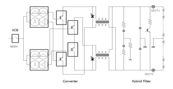
Figure 1: Principal circuit of the bending magnet power supply.
