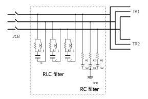
Figure 3: Filter for higher harmonic current.
