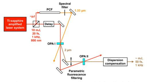
Figure 1: Non-degenerate 2 µm OPCPA system pumped by a standard Ti:Sapphire ultrafast laser system.
