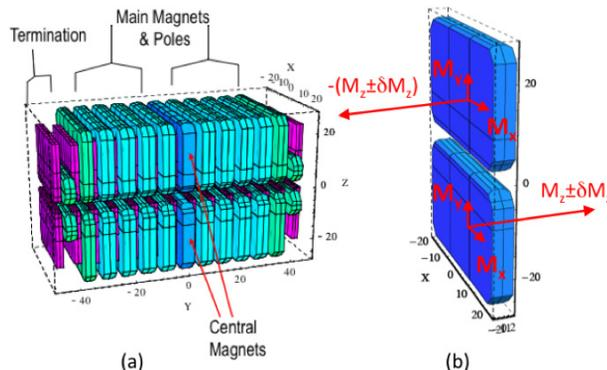
Figure 1. (a) Radia model of HPMU. (b) Central magnet pair with magnetization error components  $\delta M_z$ ,  $M_y$  and  $M_x$ .
