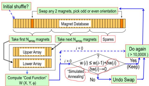
Figure 3. A simple magnet swapping algorithm.
