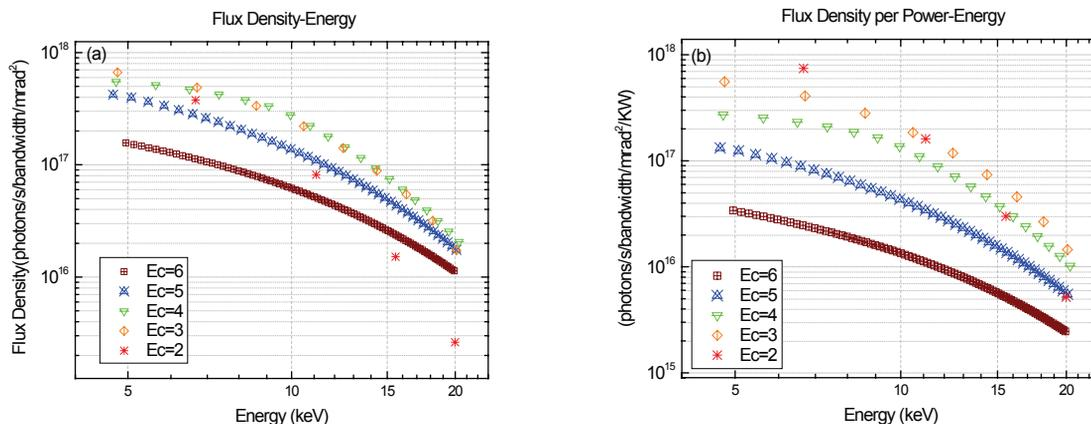
Figure 1: Maxima of harmonics within 5-20 keV are drawn with points to indicate the maximal intensity of each harmonic. Five cases of critical energy -- 2, 3, 4, 5 and 6 keV -- are shown. (a) flux density, (b) flux density per total radiation power.
