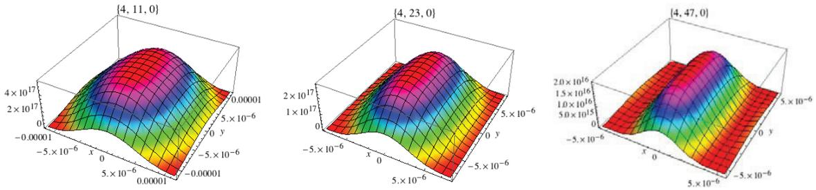
Figure 3: Patterns of the distribution of flux density in transverse directions of the e-beam. Three cases -- 11<sup>th</sup>, 23<sup>rd</sup> and 47<sup>th</sup> harmonics – with  $E_c=4$  keV in Fig. 1 are shown. The scale of transverse axis has unit rad; The plot range is the opening angle of each harmonic, which varies case by case.
