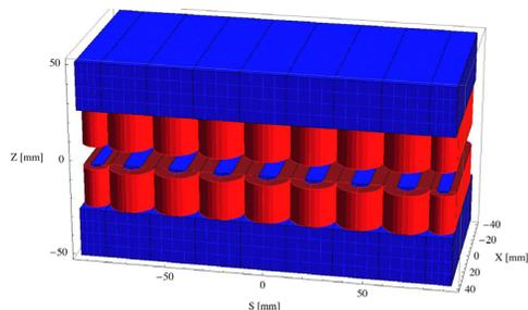
Figure 5: Magnetic model of the scw46 ID. The ID has been modelled with Radia [4].
