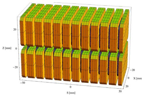
Figure 1: Magnetic model of the pmu18p5 ID. The magnet has been modelled with Radia [4].
