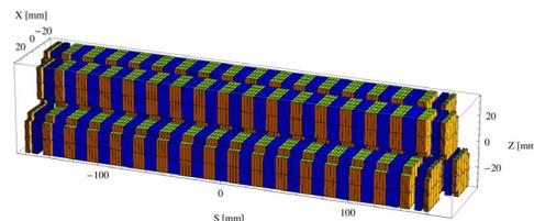
Figure 3: Magnetic model of the epu38Heli ID. The ID has been modelled with Radia [4].
