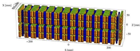
Figure 4: Magnetic model of the wig80 ID. The ID has been modelled with Radia [4].
