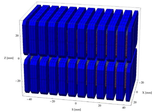
Figure 2: Magnetic model of the cpmu16 ID. The magnet has been modelled with Radia [4].
