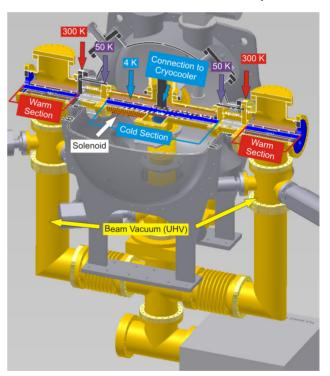
Figure 1: Sketch of the cryostat
