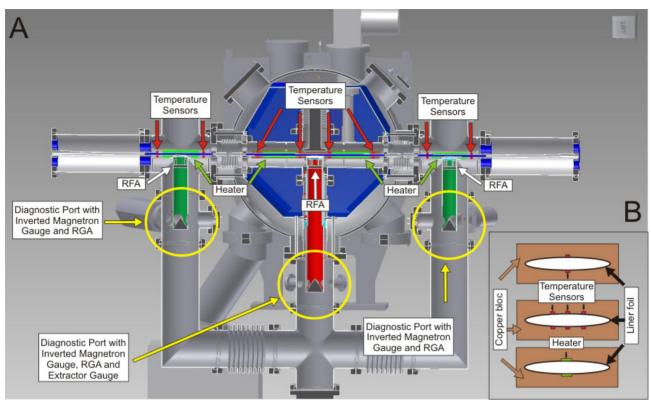
Figure 2a, b: Overview of the diagnostics installed in COLDDIAG
