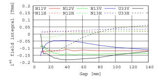
Figure 5: Residual gap dependence of vertical (solid) and horizontal (dashed) field integrals after adjustment of end poles. These kicks are compensated by corrector coils.
