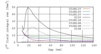
Figure 4: Second field integral rms value as function of gap, indicating the trajectory straightness. Values should be compared to the ideal trajectory rms value of 16 Tmm<sup>2</sup> related to the intrinsic oscillating motion at minimum gap.
