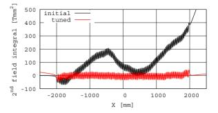
Figure 7: U33 trajectory correction.
