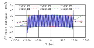
Figure 2: Vertical (solid) and horizontal (dashed)  $2^{nd}$  field integrals of U32 undulators at 9 mm gap.
