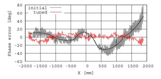
Figure 8: U33 phase error correction.
