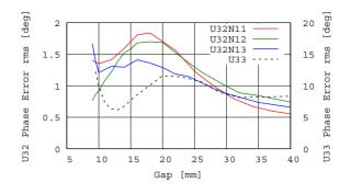
Figure 1: Gap dependence of the phase error (rms) for U32 (left) and U33 (right) undulators.
