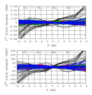
Figure 6: Transverse dependence of  $1^{st}$  (top) and  $2^{nd}$  (bottom) field integral values for different gaps measured by stretched wire (gap dependent dipole correction applied).
