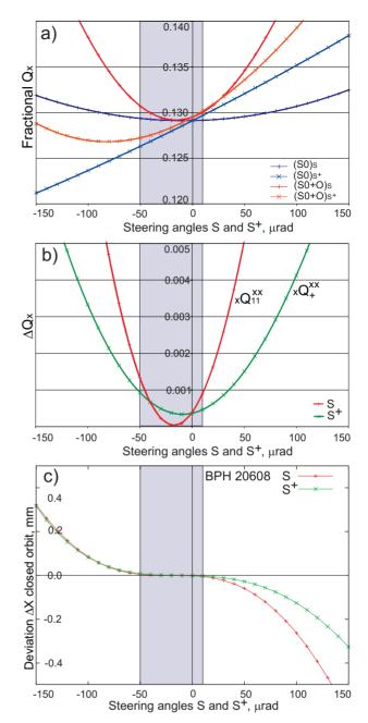
Figure 1: Simulated a) fractional part of the SPS horizontal tune vs. horizontal steering angles for only chromaticity sextupoles (blue and light blue) and with octupoles (red and orange). b) The correspondent differential tune response. c) Deviation of CO from linear response.
