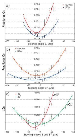
Figure 2: Measured fractional part of the SPS horizontal tune for chromaticity sextupoles switched on and octupoles on top of the chromaticity setting vs. horizontal steering angles S in a) and  $S^+$  in b). c) Differential tune response.
