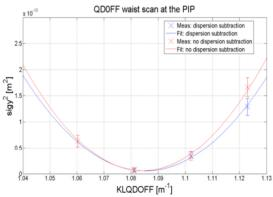
Figure 2: Vertical waist scan at IP using IPBSM and QD0FF.
