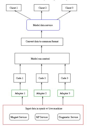
Figure 1: Data flow for model engine and service.
