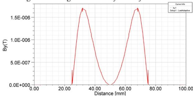
Figure 11: Y component of B for the magnet is Fig. 10.
