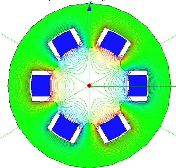
Figure 6: Flux line in a sextupole magnet.
