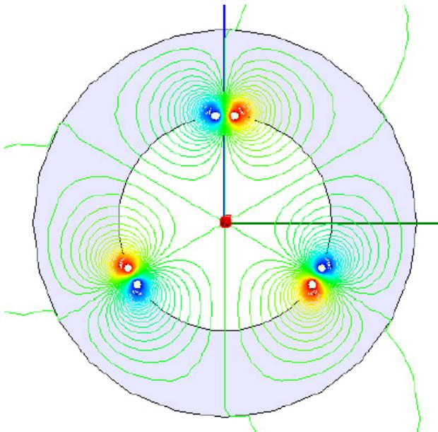
Figure 10: Magnet with tri-symmetry and flux.
