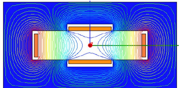
Figure 3: Quadrupole flux with a rectangular core.
