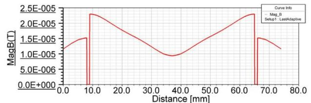
Figure 2: Magnitude B across center of aperture.
