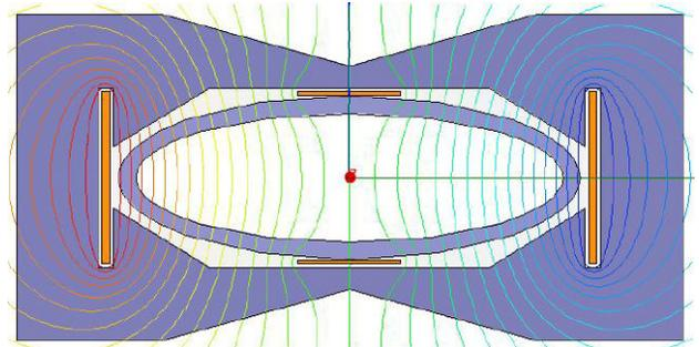
Figure 1: Dipole magnet flux line.
