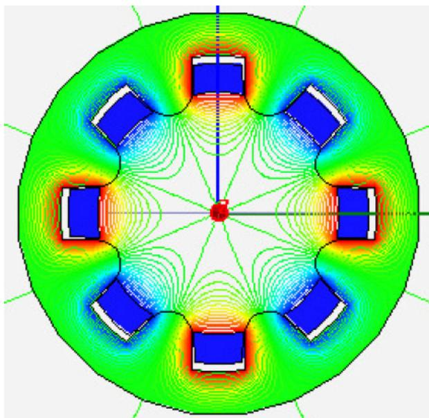
Figure 12: Octupole magnet and flux.
