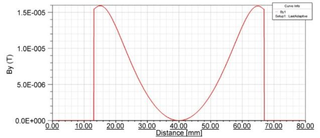
Figure 7: Y component of B for the magnet in Fig. 6.
