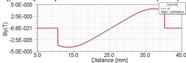
Figure 5: Y component of B for magnet in Fig. 4.
