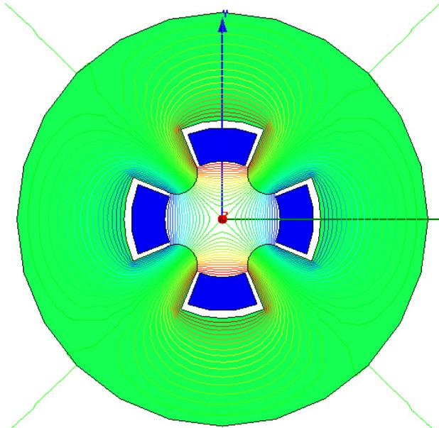
Figure 4: Quadrupole flux with circular core and pole tips.
