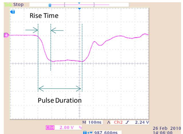
Figure 5: Typical PFN current waveform in dual one-turn coils configuration. Current monitor: Pearson-101; sensitivity: 0.01 volt/Amp.
