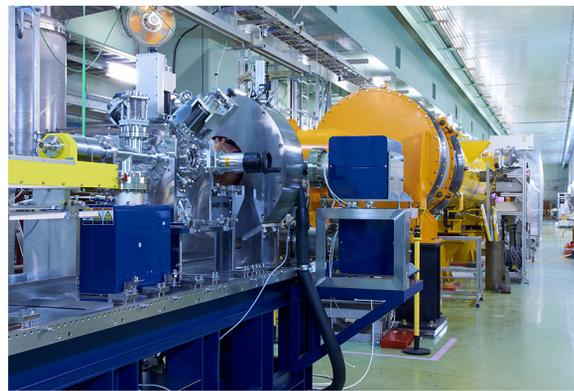
Figure 5: The L-band rf gun system at KEK-STF injector.
