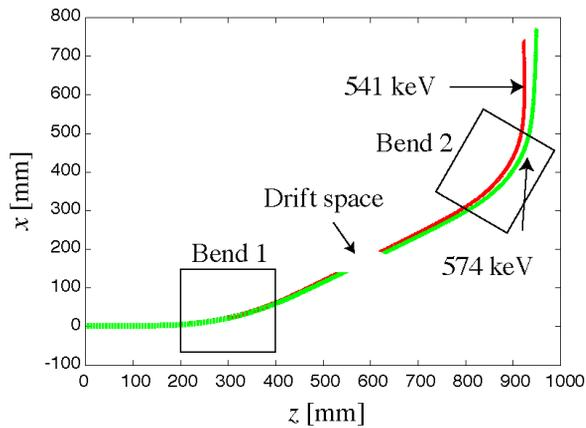
Figure 4b: the beam trajectories of proton beams with kinetic energy of 541 keV and 574 keV.
