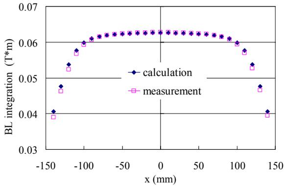
Figure 2a: A comparison between calculation and measurement values of the first dipole (BL integration, that is, the  $B_y$ -component integrated along a beam trajectory).
