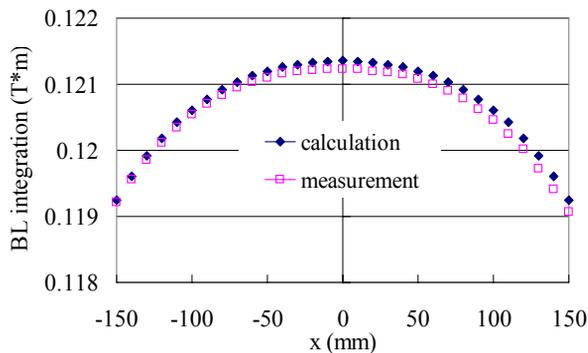
Figure 2b: A comparison between calculation and measurement values of the second dipole (BL integration of the  $B_y$ -component).
