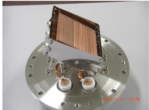
Figure 5: Analyzer detector head.
