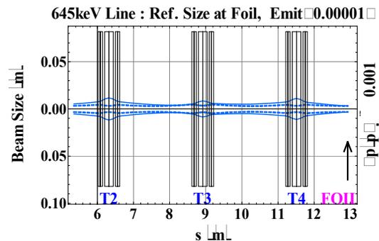
Figure 4a: The optics of beam line for the reference case. Plain and dashed lines show the horizontal and vertical beam sizes, respectively.
