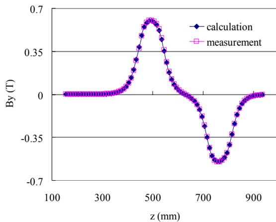
Figure 3: A comparison between calculation and measurement values of the doublet quadrupole magnets ( $B_y$ -component along an offset line by 20mm from the central trajectory).
