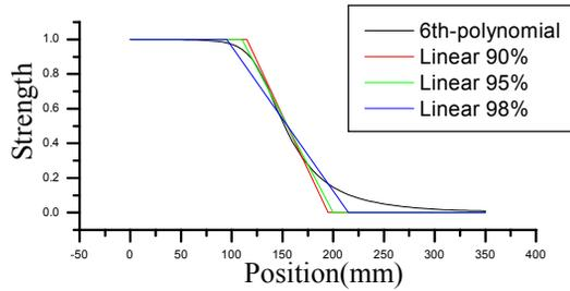
Figure 1: Different model of fringe field of quadrupole magnet.
