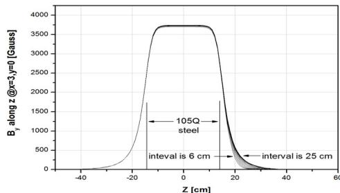
Figure 2: Influence of 130S magnet core over the fringe fields of 105Q magnet
