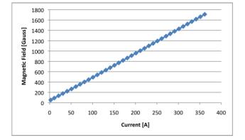
Figure 3: The center field as function as current.
