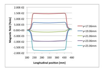
Figure 6: The field map of the quadrupole prototype.
