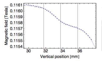
Figure 5: The magnetic field near vertical center and its polynomial fit. The fit function reads as  $B = 0.1158 - 9.859 \times 10^{-5} (y - y_c) + 1.887 \times 10^{-5} (y - y_c)^2 + 4.658 \times 10^{-6} (y - y_c)^3 - 2.278 \times 10^{-6} (y - y_c)^4 - 2.499 \times 10^{-7} (y - y_c)^5 + 4.781 \times 10^{-8} (y - y_c)^6$  Tesla, where  $y_c = 33.749$  mm. The grid lines corresponds to 33.749 mm and  $\pm 2$  mm.
