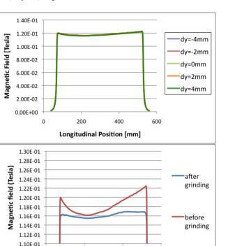
Figure 4: The longitudinal field map at different vertical position (top), the comparison of the field at y = 0 before and after the magnet pole surface is grinded (bottom).
