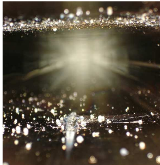
Figure 1: Impact of a 2.1 MJ beam. Over a length of about 10 cm the vacuum chamber is punctured. Metal droplets contaminate the vacuum chamber.
