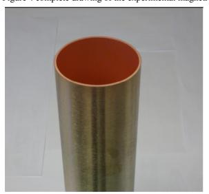
Figure 5 copper coated RHIC tube sample
