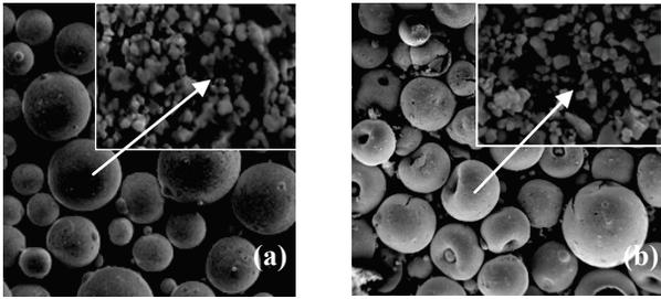
Figure 1: SEM images of NiZn (a) and MnZn powder (b). The inserts show the surface morphology of the particles.
