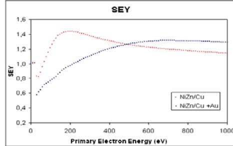
Figure 2: SEY of NiZn/Cu and NiZn/Cu coated with gold as a function of the primary electron energy.
