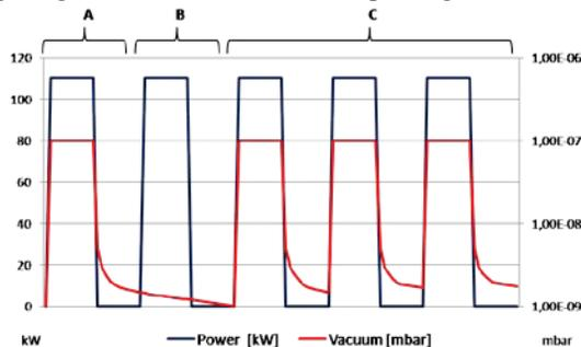
Figure 6: RF power (blue trace) and Vacuum activity (red trace) while applying several current levels along the coil.
