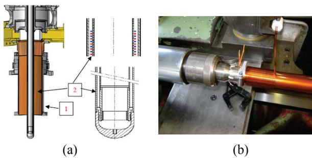
Figure 5: (a) Part of the LHC Main Coupler design. The open ended 75  $\Omega$  coaxial line under vacuum is shown. 1 is the outer conductor double walled and 2 the inner conductor copper antenna. (b) Coiling of the inner cane of the air cooling antenna.
