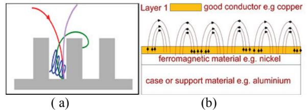
Figure 4: Magnetized surface effect on the secondary electron trajectories: (a) Magnetized rough surface and (b) Magnetized flat surface.
