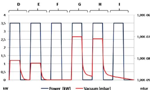
Figure 7: RF power (blue trace) and Vacuum activity (red trace) with NSNS pattern (DEF) and NNSS pattern with 2 mm spacers between each magnet (GHI).
