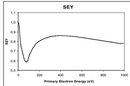
Figure 3: SEY of particulated FeSr ferrite as a function of the primary electron energy.
