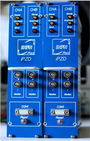
Figure 4: Two iPZD Modules. Com port is used to program the Digital Signal Controller.
