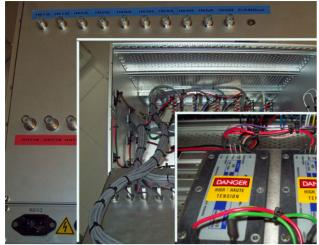
Figure 2: Piezo Control Unit back panel and insight view evidencing cabling and high voltage dc-dc converters
