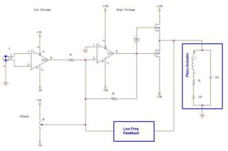
Figure 1: Conceptual Schematic
