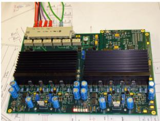
Figure 3: iPZD Module. Each module drives two independent channels.
