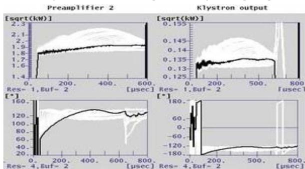
Figure 9: Reduction of peak forward power by gain scheduling during filling time.
