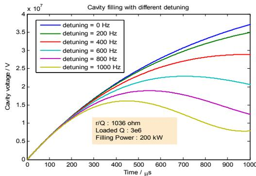
Figure 1: Cavity filling with different detuning.
