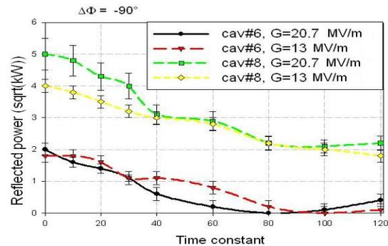
Figure 7: Minimization of reflected power.
