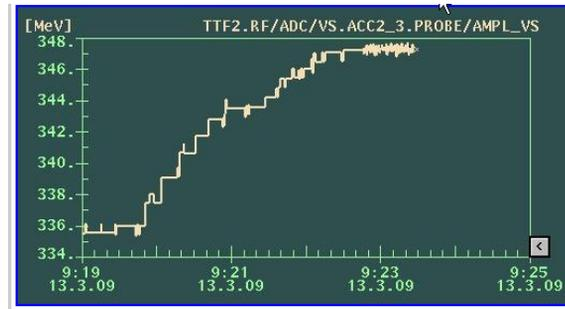
Figure 6: Energy gain increase by phase modulation.
