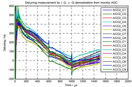
Figure 2: Detuning measurement at FLASH accelerating modules.
