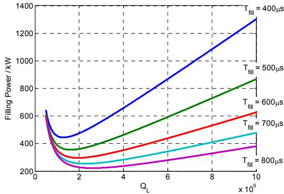
Figure 3: RF filling power for different loaded Q and filling time.
