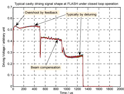
Figure 8: Typical cavity driving signal at FLASH under closed loop operation.
