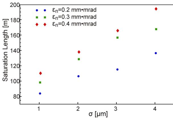
Figure 2: Dependence of saturation length on beam rms length at three values of beam normalized emittance.
