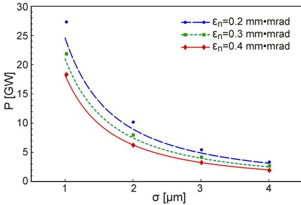
Figure 1: Dependence of saturation power on beam rms length at three different values of beam normalized emittance. (points – simulation results, lines – analytical scaling).
