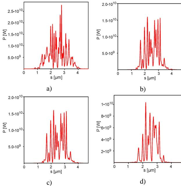
Figure 5: Power distribution along the bunch at the saturation point for the following values of energy spread: 1.4 (a), 2.3 (b), 3.3 (c) and 4.3 MeV (d).
