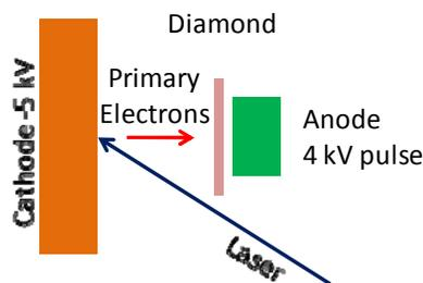
Figure 1: Amplified Photocathode
