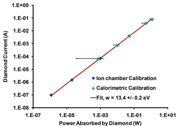
Figure 4: Linearity of current in diamond with respect to absorbed x-ray power.
