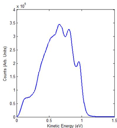
Figure 5: Electron energy spectrum emitted from a hydrogen-terminated, boron-doped diamond.
