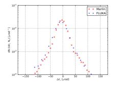
Figure 2: The distribution of change in proton direction after scattering through 0.5 m of Copper collimator.
