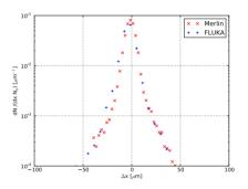
Figure 1: The distribution of change in proton position after scattering through 0.5 m of Copper collimator.
