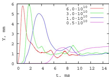
Figure 4: Evolution of the beam offset amplitude for  $\text{Ar}^{18+}$ .  $E = 11.4 \text{ MeV/u}$
