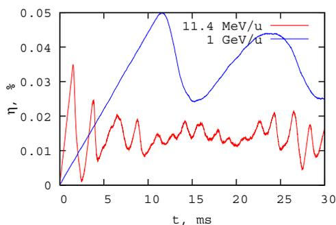
Figure 3: Evolution of the neutralization degree for  $\text{Ar}^{18+}$  for SIS-18 injection and extraction energies.  $N_{\text{beam}} = 2.0 \cdot 10^{10}$
