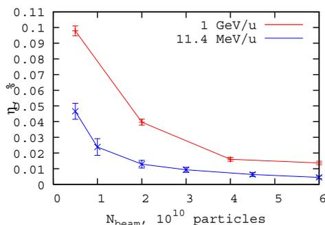
Figure 5: Steady-state neutralization degree for  $\text{Ar}^{18+}$  as a function of number of particles for injection and extraction energies.
