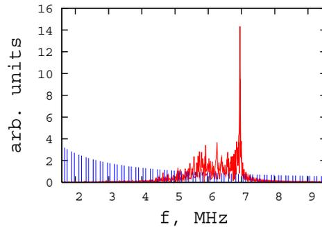
Figure 2: Electron transverse spectrum (red) and transverse Schottky spectrum (blue) for  $U^{73+}$  and  $N_{beam} = 10^{10}$ .
