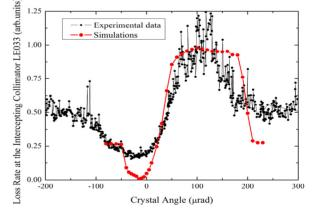
Figure 2: Results of angular scan with 8-strip vertical crystal. Red line is for computer simulations results.
