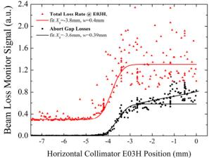
Figure 3: Collimator scan with crystal set at the channeling angle. Solid lines are for "erfc" fit of the data.
