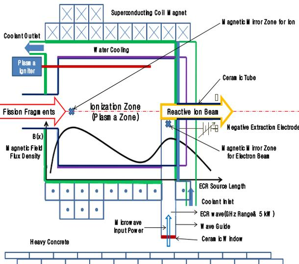
Figure 2. Physics Design of Electron Cyclotron Resonance Source
