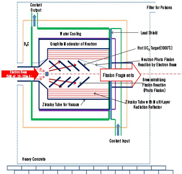
Figure 1. Physics Design of ECR Target (Fission) Chamber with SC Coil
