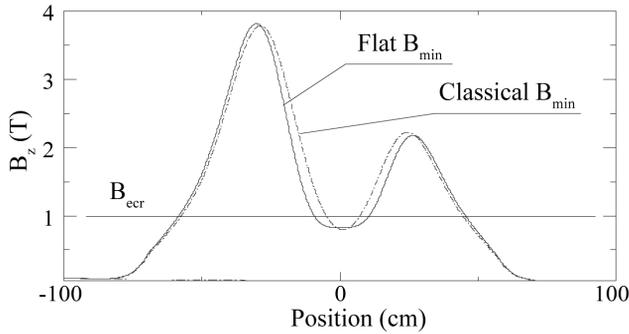
Figure 2: Typical axial magnetic field strength.
