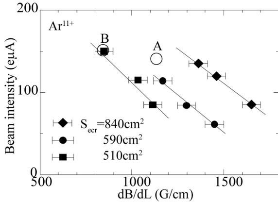
Figure 6: Beam intensity of  $\text{Ar}^{11+}$  ions for several average magnetic field gradient at ECR zone.
