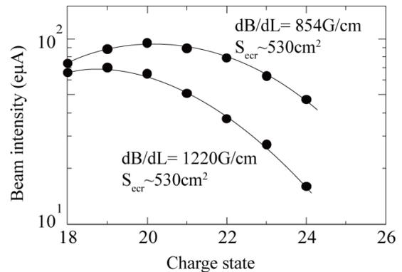
Figure 4: Charge distributions of Xe ions for the average magnetic field gradient  $dB/dL \sim 850$  and  $1220G/cm$ .
