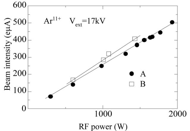
Figure 7: Beam intensity of  $\text{Ar}^{11+}$  as a function of RF power at two conditions (A and B).
