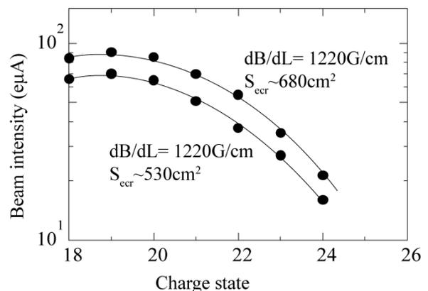
Figure 5: Charge distribution of Xe ions for the ECR surface size of 686 and 530  $cm^2$ .
