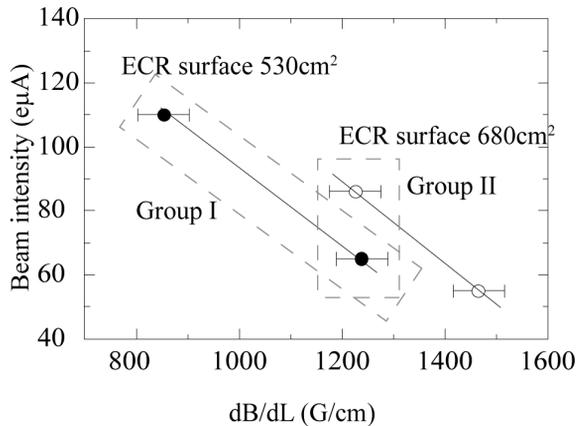
Figure 3: Beam intensity of  $Xe^{20+}$  ions for several average magnetic field gradient at ECR zone.
