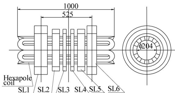
Figure 1: Schematic drawing of the SC-coils of RIKEN SC-ECRIS.
