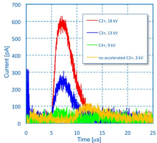
Figure 6: Pulse structure of analyzed beam from the linac.
