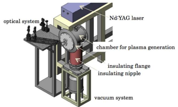
Figure 2: A schematic drawing of the two-beam type laser ion source with DPIS.
