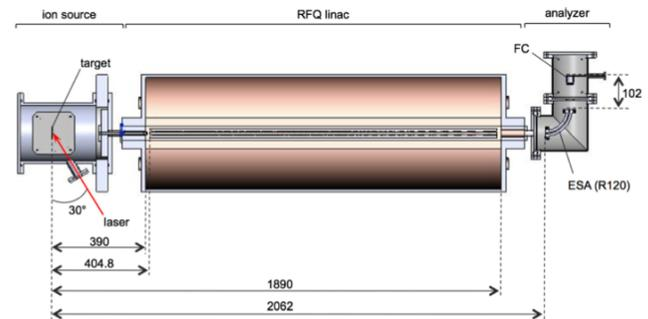
Figure 3: A layout of acceleration test for two-beam type IH-RFQ
