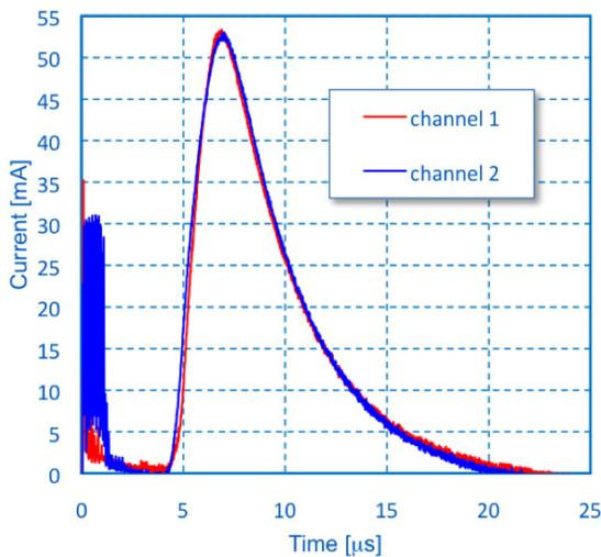
Figure 5: Output beam's waveforms from each channel. This data are averaged over 8 laser shots.
