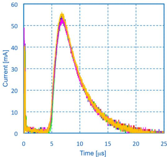
Figure 4: Current waveforms outputted from beam channel 1 in the superposition of 5 laser shots.
