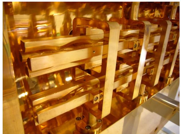
Figure 1: A photo of the two-beam type IH-RFQ linac.
