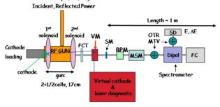
Figure 1. Photo injector layout: symbols explanation is given in the text.
