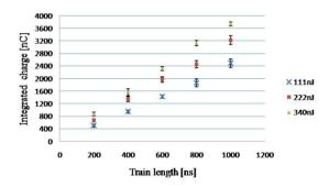
Figure 2: Integrated charge as function of train lengths for three different laser pulse energies: 111, 222 and 340 nJ. Laser transverse size  $\sigma$ ~0.3mm.
