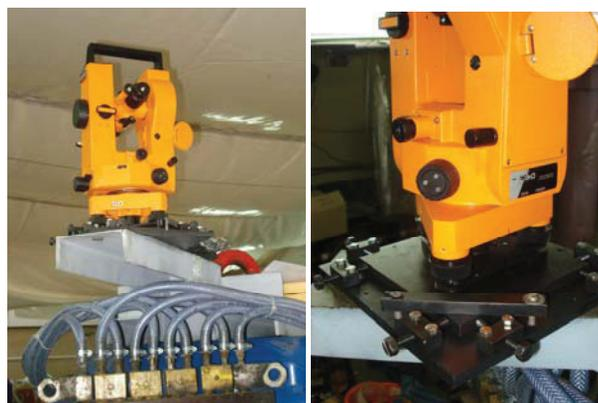
Fig. 5. View of a theodolite mounting at a NESTOR bending magnet.
