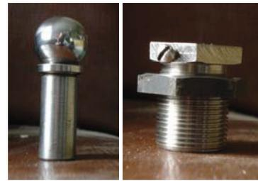
Fig. 2. An example of ball survey target and fixing socket.
