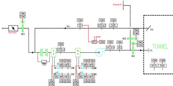
Figure 5: Structure of the tunnel AHU system.
