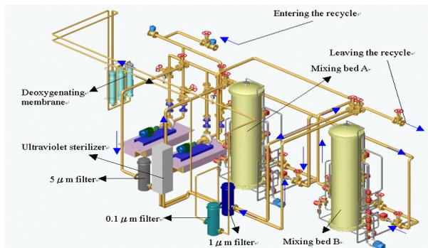
Figure 4: Structure of water treatment.
