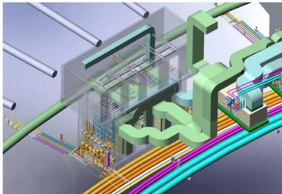
Figure 7: Arrangement of air ducts near the CIA.
