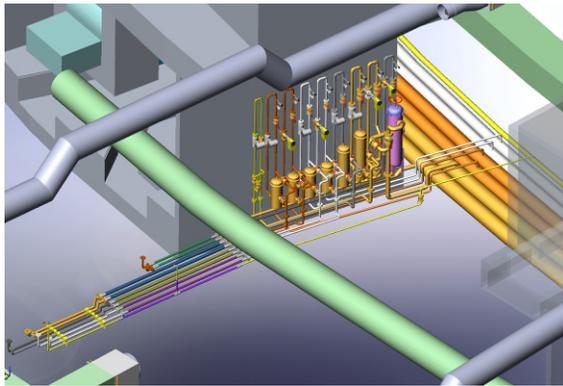
Figure 3: Manifold arrangement near a CIA.
