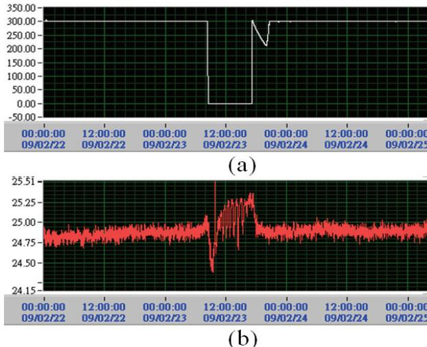
Figure 3: Beam current (mA) (a) and temperature history during machine shutdown after temperature control improvement (b).
