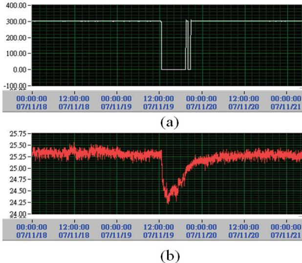
Figure 2: Beam current (mA) (a) and temperature history during machine shutdown before temperature control improvement (b).
