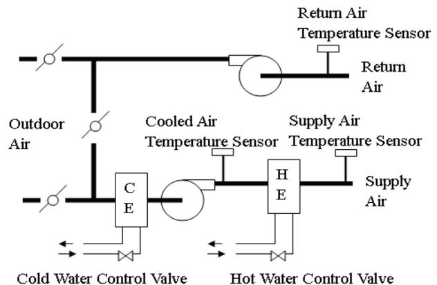
Figure 1: Control system of the AHU.
