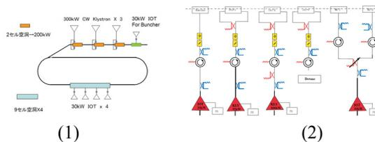
Figure 1: RF layout. (1) shows 65MeV plan of cERL and (2) shows the 35MeV reduced version.
