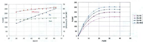
Figure 2: Characteristics of 300-kW klystron. Left: Applied voltage vs. output power (black), gain (green) and efficiency (red). Right: Input power vs. output power in various applied voltage.
