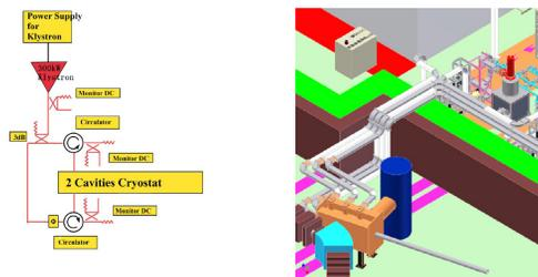
Figure 3: Left: Block diagram of the RF system for the 2-cavities cryostat. Right: Power distribution layout of the injector of cERL.
