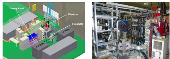
Figure 4: Left: Schematic drawing of the test station. Right: Photograph of the RF source in the PF Power Supply Hall.
