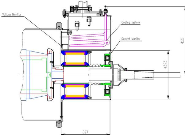
Figure 7: New design of CM, left side gun tank of klystron, on the right HV cable connection.
