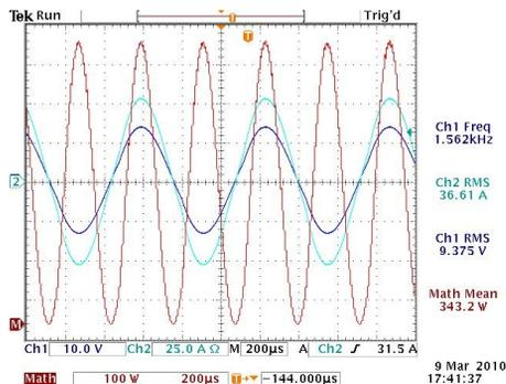
Figure 3: Waveforms of voltage and current on the cathode heater of TH-1802.
