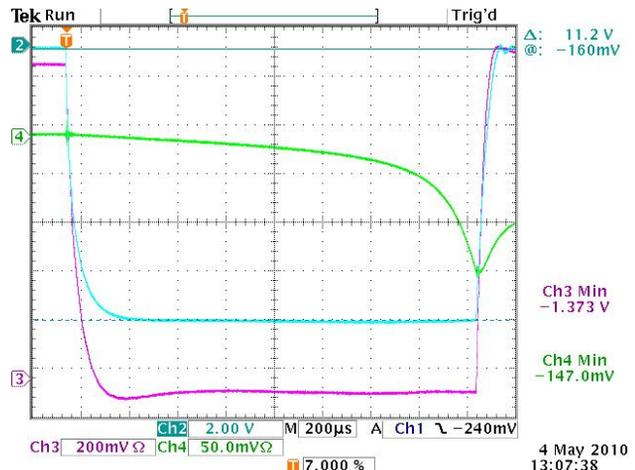
Figure 5: Pulse shape of cathode current, high voltage and leakage current measurement.
