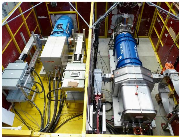
Figure 1: Multibeam klystrons test stand in DESY, left Toshiba MBK connected directly to the pulse transformer tank, on right side Thales MBK with CM connected to the pulse transformer through HV cable.
