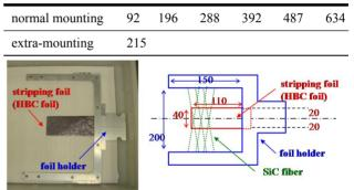
Figure 1: Schematic diagram of the operational foil mounting on the C-shaped holder.
