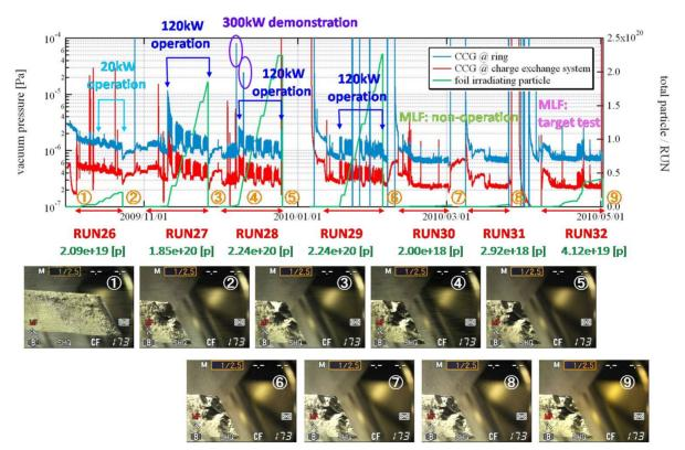
Figure 8: Trends of outgassing from the foil and the deformations on the foils during the beam irradiation. The upper graph plots the vacuum pressure measured by the CCG around the stripping foil and the total irradiated particle every run cycle. The lower photos show the deformations of the HBC foils during the beam irradiation.
