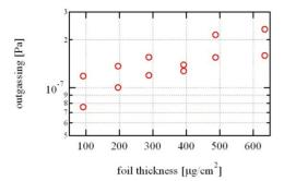
Figure 7: Pressure increments of the vacuum right after the first beam irradiation and 40 minutes later as a function of the foil thickness measured with beam.
