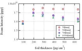
Figure 6: Typical results of the charge exchange efficiency and beam loss caused by the foil scattering as a function of the foil thickness.
