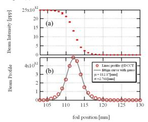
Figure 3: Typical result of the foil scanning. (a) shows the circulating beam intensity as a function of the foil position. (b) is the injection beam profile obtained by differentiating (a).
