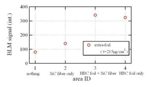
Figure 5: Measurement results of the SiC fiber effect.
