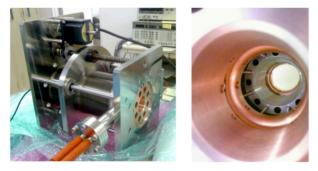
Figure 3: Pre-buncher chamber and its drift tubes.
