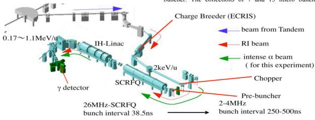
Figure 1: Layout of TRIAC with pre-buncher.
