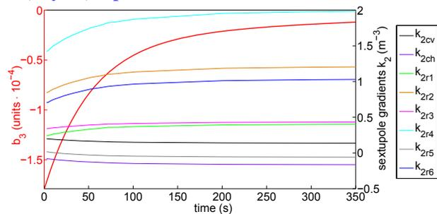
Figure 4: Estimated  $b_3$  decay together with the dynamic sextupoles strengths proposed for its compensation.
