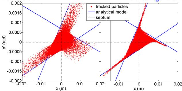
Figure 3: Phase-space plots of 1000 particles tracked for 100 turns. The left figure shows the particles before and the right one after the compensation by means of a new set of optimized strengths for the 2+6 families of sextupoles.
