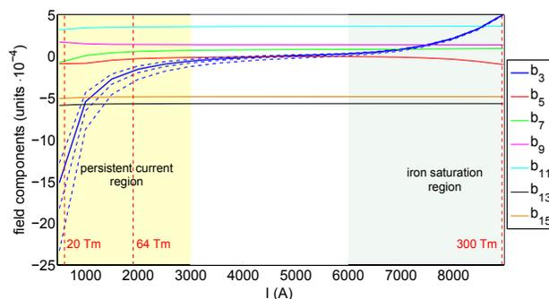
Figure 2: ROXIE simulations for the allowed field components of the SIS300 dipoles up to  $b_{15}$ . The field component  $b_3$  is plotted in blue for different filament diameters (2, 2.5, 3.5 and 4  $\mu\text{m}$ ). The absolute value of  $b_3$  increases with the thickness of the filaments at low fields. The thick blue line is used as a reference value (2.5  $\mu\text{m}$ ) in the text.
