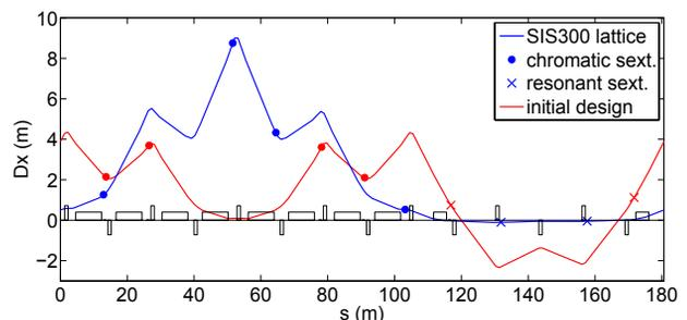
Figure 1: Dispersion functions of the modified and the initially proposed SIS300 lattice (WP = 13.31, 9.27), plotted for 1 sector of the ring. Dipoles and quadrupoles are depicted in the figure while the chromatic and resonant sextupoles are indicated along the dispersion functions.
