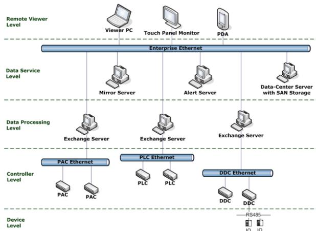
Figure 3: Network architecture of the control and archive system.
