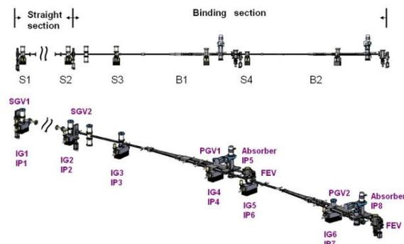
Figure 1: Layout of a typical vacuum system for one period including straight section and bending section.
