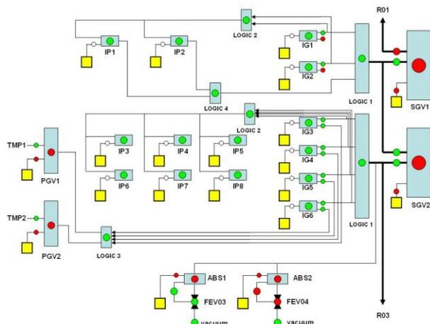
Figure 4: Layout of the vacuum-interlock control panel as SR02 section. The circle is a light indicator and the empty square is the push-button. The green, red and red flash lamps indicate the status of ready (open), fault (close) and not ready, respectively.
