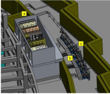
Figure 2: Geometry of (a) control instrument area (CIA), (b) trenches, and (c) one unit cell.
