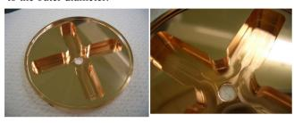
Figure 3: Typical damped cell of TD18 structure (left) and detailed shape near iris of TD18 structure (right).
