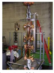
Figure 7: Two structures and their vacuum container.
