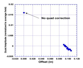
Figure 5: Electric Quadrupole field component at a radius of 3 mm.
