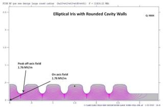
Figure 2: SUPERFISH simulation of complete RF gun.
