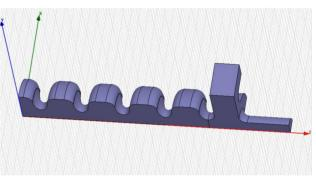
Figure 3: RF Gun geometry use in HFSS.
