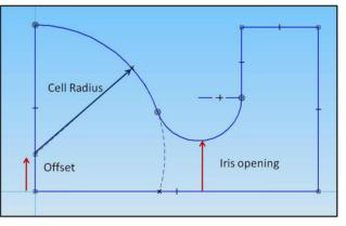
Figure 4: Coupling Cell transverse profile.
