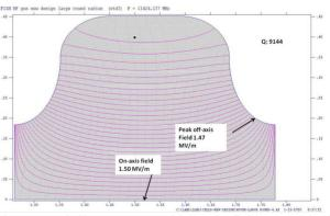
Figure 1: Cell geometry with peak fields at cathode (cavity centre) matched to peak iris fields.
