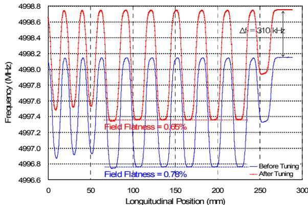
Figure 5: The result of the bead test. The blue line test is conducted before tuning, and the red line test is conducted after tuning.
