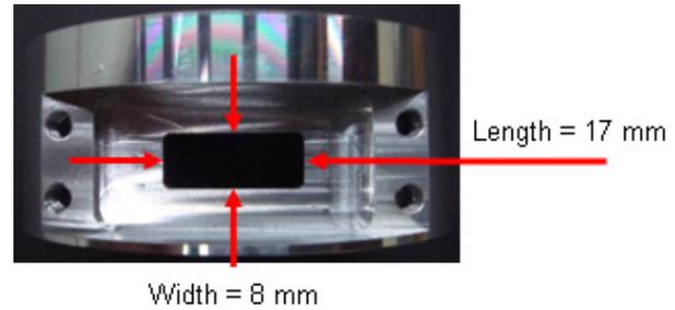
Figure 3: The RF input coupler of the coupler cell.
