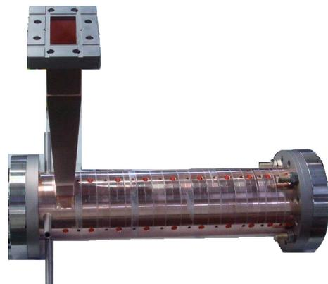
Figure 4: The actual accelerating structure with the OFHC copper.
