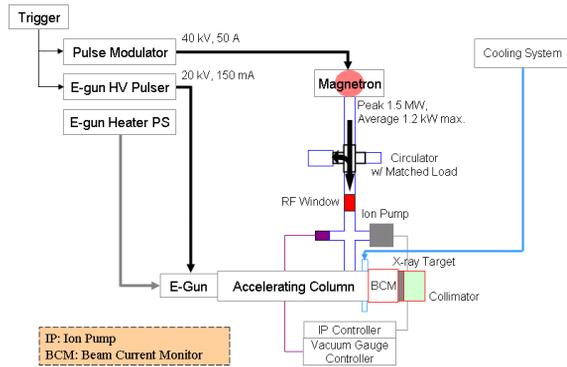
Figure 1: The schematic diagram of accelerator system.
