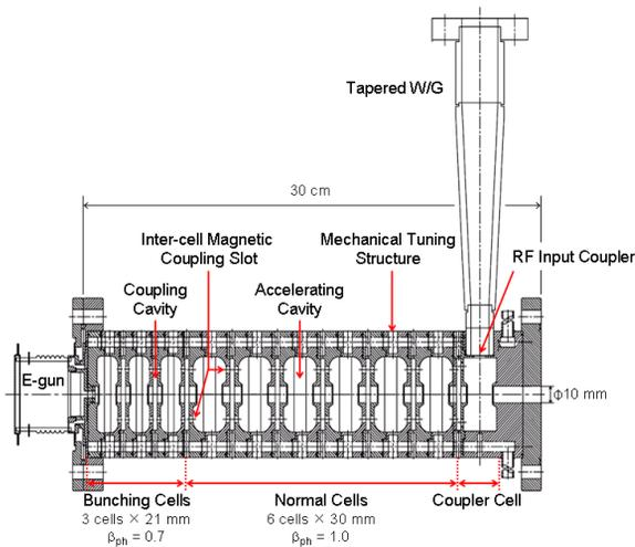
Figure 2: The cross-sectional view of the accelerating structure. The inter-cell magnetic coupling slots are skewed to this plane.
