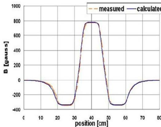
Figure 2: Magtic flux profile of the triplet [2]
