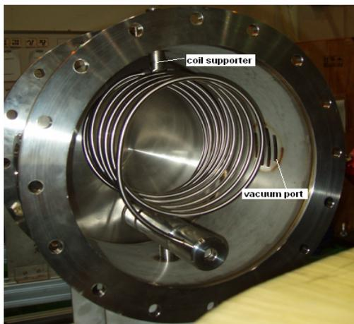
Figure 4: Picture of the cavity under construction
