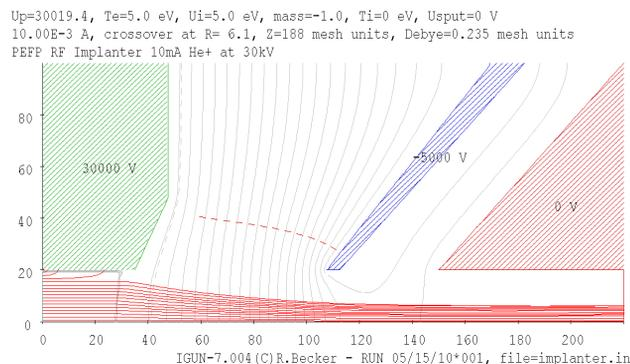
Figure 1: IGUN simulation for the ion source
