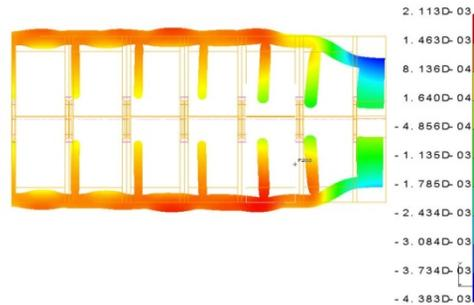
Figure 5: Thermal deformation of collinear load with Kanthal coatings.
