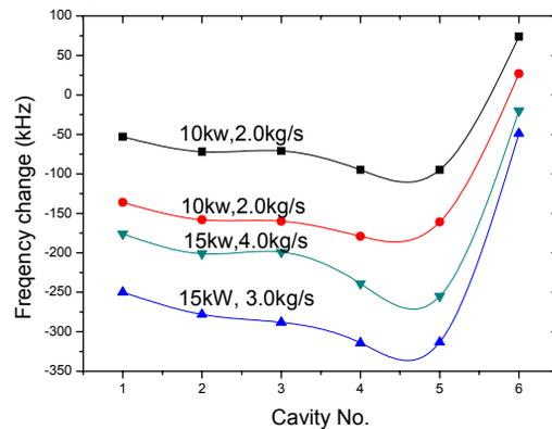
Figure 6: Frequency change of collinear load with Kanthal coatings.
