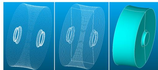
(a) nodes (b) section curves (c) deformed cavity
