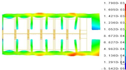
Figure 8: Thermal deformation of collinear load with FeSiAl coatings.
