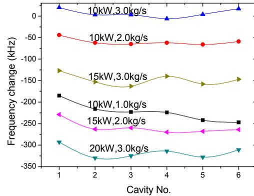
Figure 9: Frequency change of collinear load with FeSiAl coatings.
