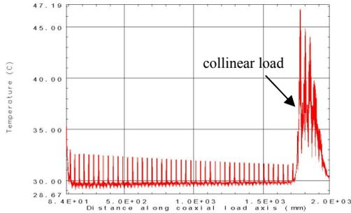
Figure 3: Axial temperature of accelerating tube with one-way cooling structure.
