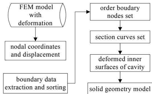
Figure 1: Flow chart of 3D reconstruction.
