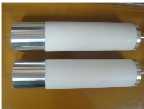
Figure 7: A pair of probes for the diagnosis of the individual cells.
