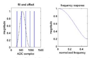
Figure 5: Time filter (left) and corresponding frequency response of the BPM (right).
