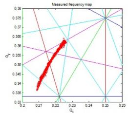
Figure 3: measured FM for the Diamond storage ring.
