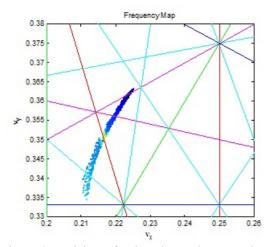
Figure 4: model FM for the Diamond storage ring
