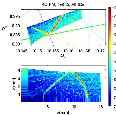
Figure 6: 2000 turns, 4D, on momentum frequency map for the bare lattice with all the IDs using the KMM and the theoretical field. Beta beating and working point change have not been corrected.
