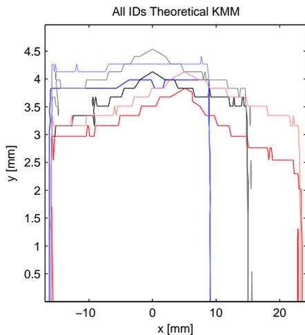
Figure 5: 500 turns, 4D, on and off momentum dynamic aperture for the bare lattice with all the IDs using the KMM and the theoretical field. Beta beating and working point change have not been corrected. Notice that the left side is limited by the septum.
