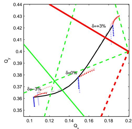
Figure 4: tune shifts with amplitude (red points for up to 16 mm horizontally and blue points for up to 4.5 mm vertically) and with energy (black lines from -3% to 3%) for the unperturbed (light colors) and the lattice with all IDs (KMM with simulated field). Red and green lines represent 3rd and 4th order resonance respectively. Beta beating and working point change have been corrected.
