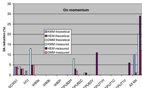
Figure 1: On momentum Dynamic aperture reduction ratio (%) for every IDs setting.
