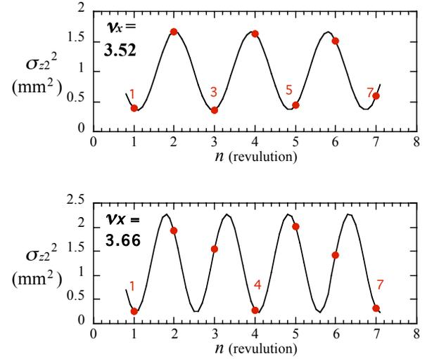
Figure 1: Bunch lengthening by a betatron motion calculated from Eq. (9). In the experiment at UVSOR-II [12] the strong CSR was observed at the 1st and the 3rd turn for  $\nu_x=3.52$ . The CSR was strong at the 1st and the 4th turn for  $\nu_x=3.66$ . It was clear that the strong CSR was observed when the bunch lengthening was small. It suggests that if  $\Delta\psi_{21}$  were not  $1.22\pi$ , the variations of CSR power were not clear.
