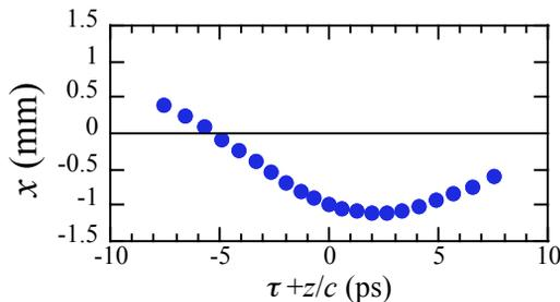
Figure 2: Bunch shape of the injected beam at a half synchrotron oscillation period after the injection. The 21 points indicate electrons, which had been equally spaced by 1 ps at the injection. The appropriate betatron phase was chosen so that the density enhancement took place at the bunch centre. The horizontal chromaticity was set at twice of the normal operation value.
