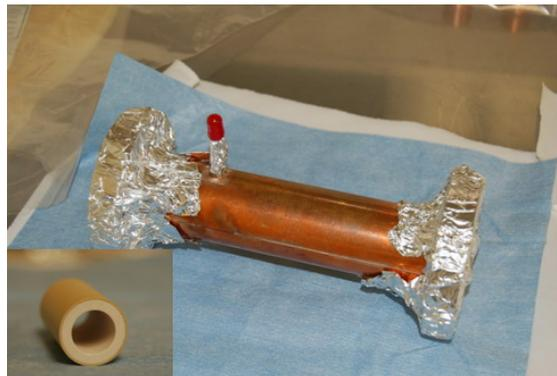
Figure 2: The finished tunable standing wave DLA structure.  $b_0=4.79\text{mm}$ ,  $b_1=6.99\text{mm}$ ,  $b_2=7.49\text{mm}$ , referring to Fig.1.
