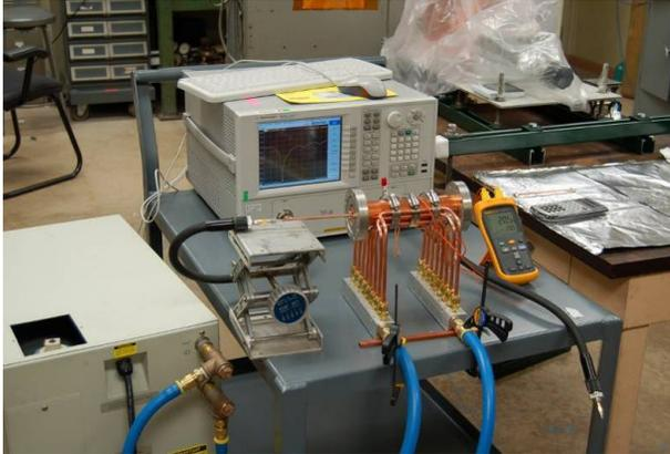
Figure 3: Setup for bench testing the tunable standing wave DLA structure.
